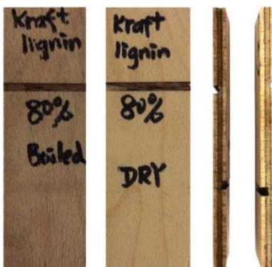
Figure 1 – Plywood panels bonded with adhesive made with dry bio-oil from Kraft lignin pyrolysis.
