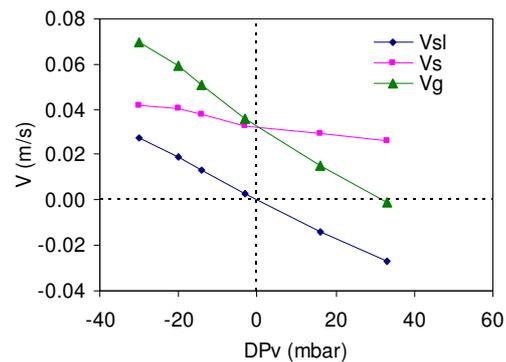
Figure 3: The change of the interstitial velocities in the standpipe due to the change of the standpipe pressure drop with  $U_{IV} = 0.2$  m/s and  $G_s = 35 - 64$  kg/m<sup>2</sup>.s (equivalent to variation of  $V_s$ ).
