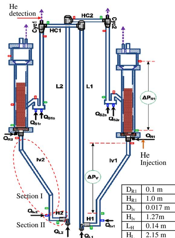
Figure 1: The scheme of the CLC cold flow prototype. Different Helium injection and detection positions are indicated in the figure.
