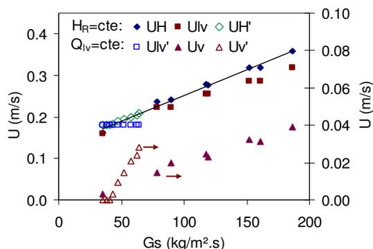
Figure 4: The variation of the solid flux versus the measured gas flow velocity in the L-valve for two experimental series: the change in external L-valve aeration with the fixed solid height ( $\diamond$ ,  $\blacksquare$ ,  $\blacktriangle$ ) and the variation of the pressure drop in the standpipe with fixed external aeration ( $\diamond$ ,  $\square$ ,  $\Delta$ ).
