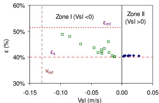
Figure 5: The experimental results of the variation of the average voidage of moving solid bed in the standpipe of the L-valve.
