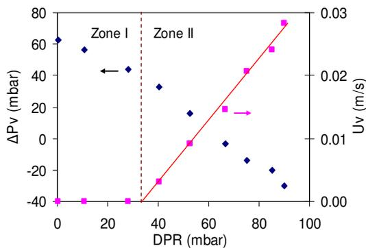
Figure 2: The effect of the reactor pressure drop on the pressure drop and the gas flow in the vertical section of the L-valve with  $U_{IV} = 0.2$  m/s.
