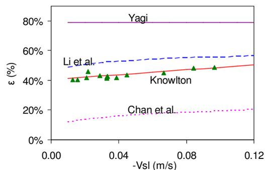
Figure 6: The experimental results of variation of the voidage of the moving solid bed in the standpipe of the L-valve compared with the literature correlations.
