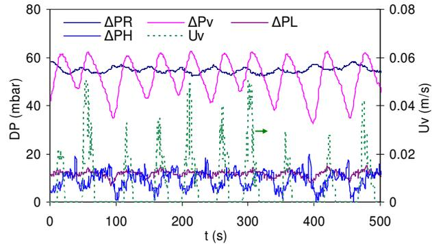
Figure 7: Oscillatory operation of L-valve in limiting condition of  $U_{iv} = 0.416$  m/s.
