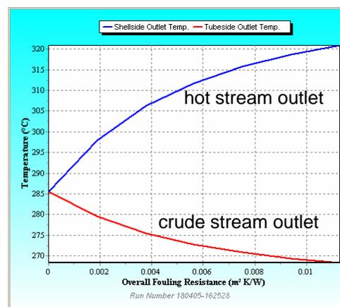
Figure 9 Thermal response of first design to fouling.
