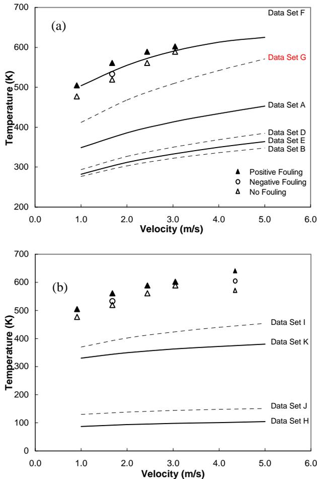
Figure 4 Threshold loci obtained from (a) pilot plant testing and (b) refinery monitoring, plotted for a standard tube size, by Yeap (2003). Symbols show Knudsen *et al.*'s data; set G is that of Srinivasan and Watkinson (2005).
