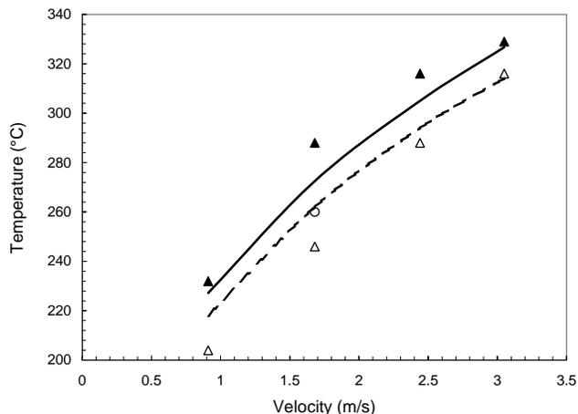
Figure 3 Pilot plant data of Knudsen *et al.* showing fouling threshold (surface temperature *v.* mean flow velocity) in an Alaskan crude oil (after Yeap *et al.* (2004). Filled symbols, fouling; open symbols, no fouling. Threshold models: Equation [3], dashed line, Equation [4] solid line.
