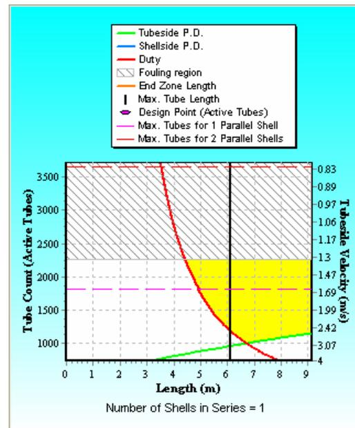
Figure 13 Parameter plot for 6 tube-pass design
