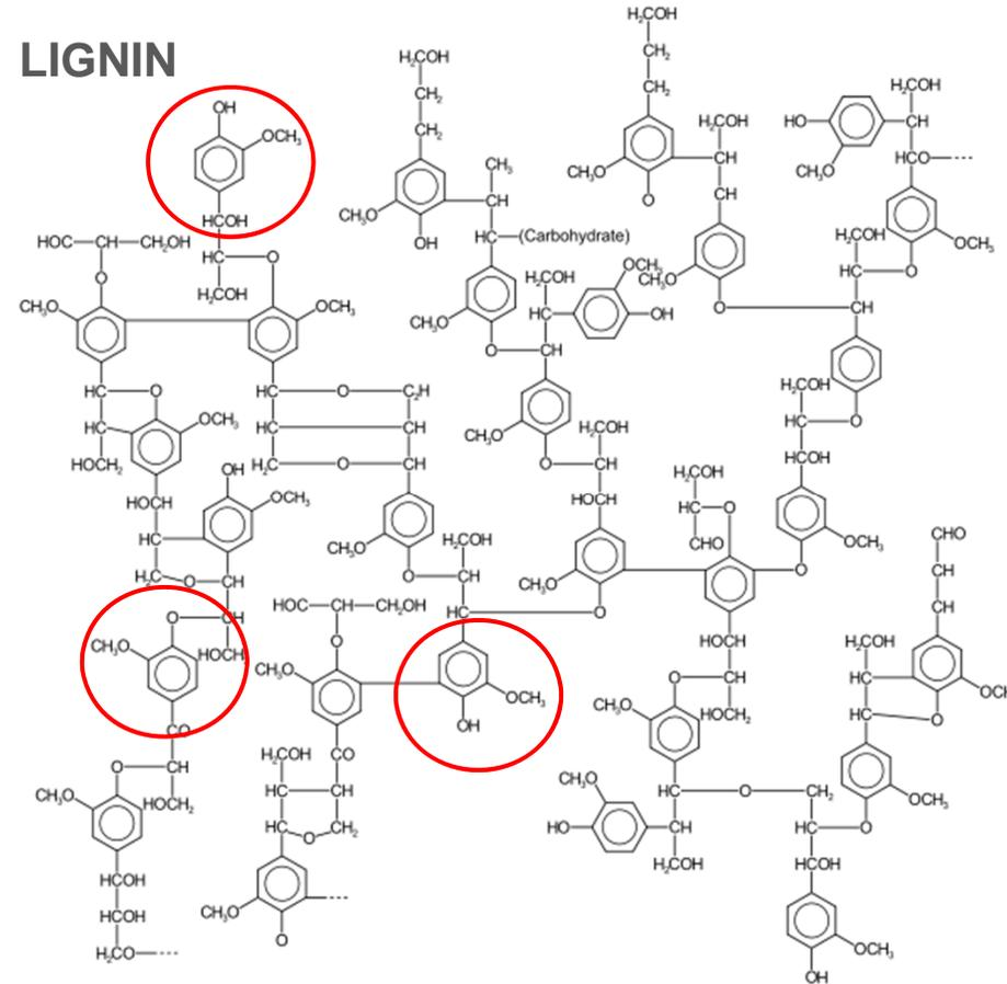
Thermal degradation → Mono-lignols: up to 15 % of bio-oil mass.
