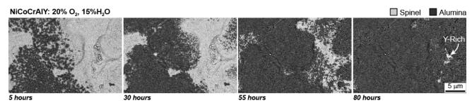
Figure 2 – A "timelapse" of NiCoCrAIY TGO (20%  $O_2$ , 15%  $H_2O$ ) from 5 to 80 hours. All backscatter images (5kV) were taken at the same site with 25 hours of oxidation (plus ramping times) separating them.
