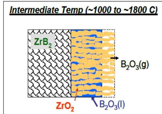
Porous ZrO<sub>2</sub> – partially filled
