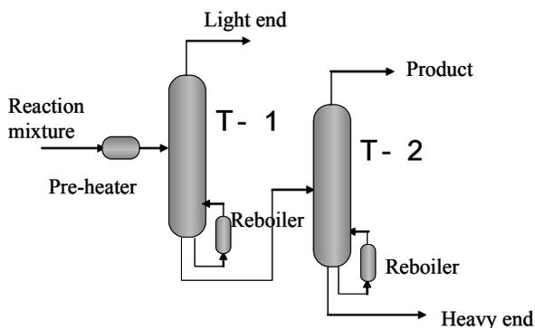
Figure 1. Distillation process flow of the plant.
