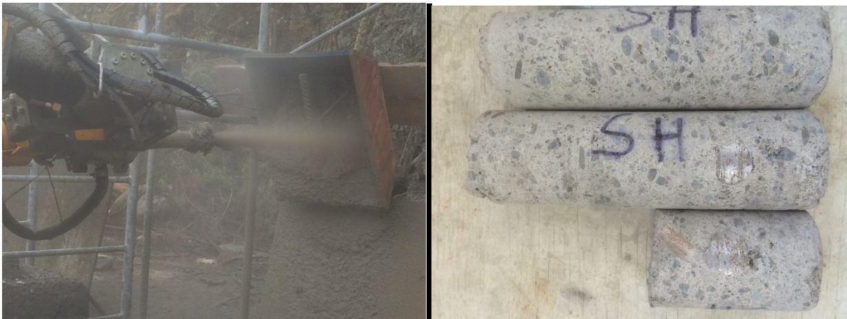
Fig. 5 Nozzleman qualification shooting with FRS for a section of lattice girder. Note that robotic sprayer shot macrosynthetic fiber reinforced wet-mix with 6% accelerator. Cores show shotcrete consolidated properly around the reinforcement.
