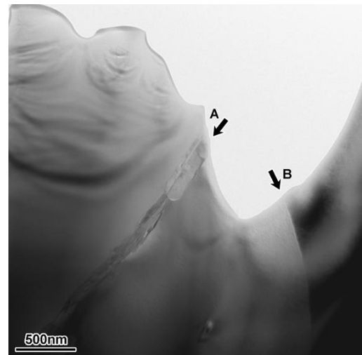
Figure 1 TEM bright field image showing secondary phase due to discharging in BaTiO 3 .
