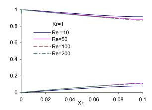
Figure 2 Longitudinal variation of the hot and cold fluid mean temperature
