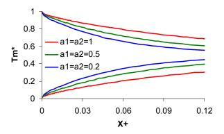
Figure 3 Longitudinal variations of the mean temperatures of hot and cold fluids for  $K_r = 100$
