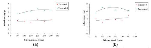
**Fig.5:** Adsorbencies on untreated and pretreated wheat straw (a) diesel and (b) crude oil spills on seawater under the effect of stirring.
