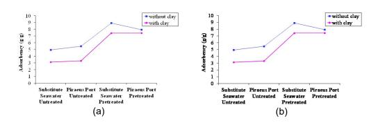
**Fig. 4:** Adsorbencies on untreated and modified wheat straw of (a) diesel and (b) crude oil spills with or without clay on substitute seawater and seawater.
