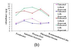
**Fig. 6:** Adsorbencies on untreated and modified wheat straw of (a) diesel and (b) crude oil spills with or without dispersant on freshwater, substitute seawater, seawater, stream water and lake water.
