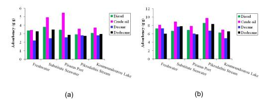
**Fig. 3**: Adsorbencies of diesel, crude oil, decane and dodecane (a) on untreated and (b) on modified wheat straw; hydrocarbon spill on freshwater, substitute seawater, seawater, stream water and lake water.
