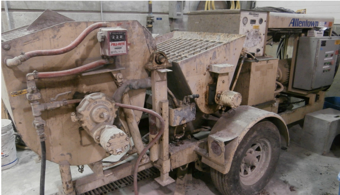
Figure 6. Allentown/Putzmeister Powercreter 10 wet-mix process shotcrete pump
