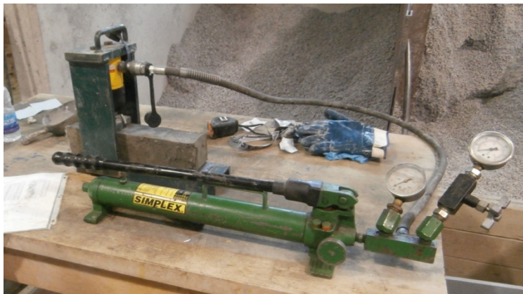
Figure 8. End Beam Test setup
