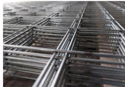
Stainless steel mesh as reinforcement
