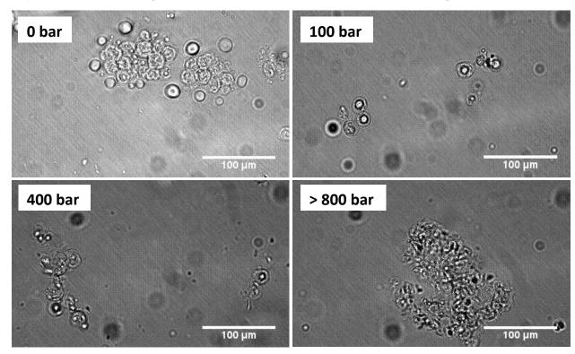
Higher levels of lipid contamination at increased homogenisation pressures
