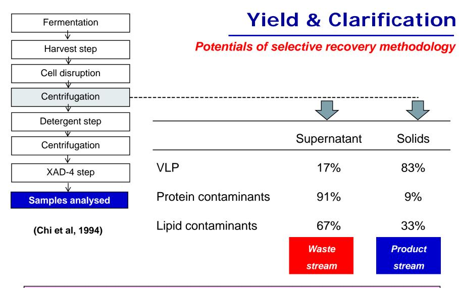
Recovery of VLP from solids fraction allows removal of bulk contaminants with minimal product loss
