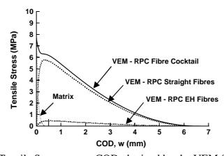
**Figure 5.** Tensile Stress versus COD obtained by the VEM for Beam 7.
