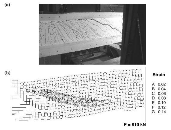
**Figure 7.** Shear cracking of RPC Beam 7 (a) Experiment; (b) FEM.
