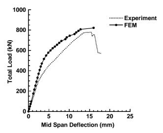
**Figure 6.** Load versus midspan displacement for Beam 7.
