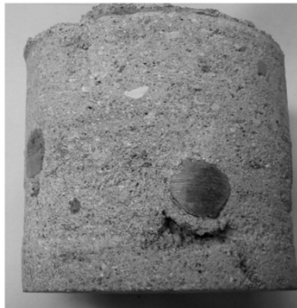
Dry-mix shotcrete, intersection #4 bars, mid size void too large to be a Core Grade #2.
