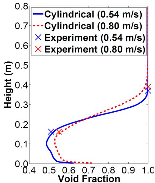
Optical probe measurements
