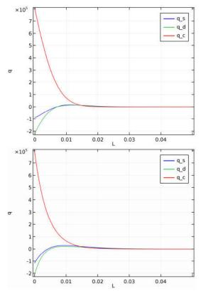
(a) Variable porosity (b) Constant porosity Fig. 3: Effect of the porosity on the heat flux in the *x* direction  $(A_p=0.9, B_p=-0.3)$
