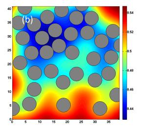
Figure 1 – Longitudinal elastic modulus as a function of the location within a fiber tow
