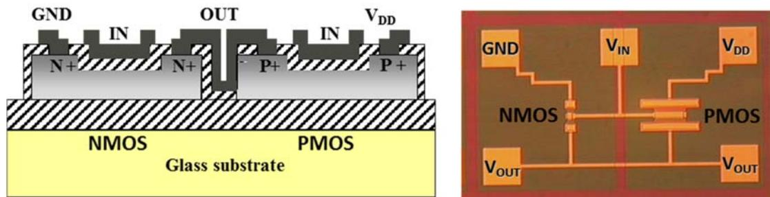
Figure 5. CMOS like TFT inverter involving solid phase crystallization of *in-situ* doped LPCVD amorphous silicon [24]. Schematic cross-section, on the left, and top-view from a microscope of the final device, on the right.
