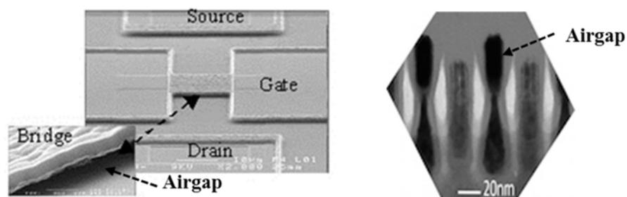
Figure 6. (left) Airgap TFT (After F. Bendriaa *et al.*) and (right) airgap FinFET (After Ed Korczynski). For both cases, the leakage current between gate contact and channel region is minimized. In the SGFET, the airgap zone can be functionalized and can act as a high sensitive sensor.
