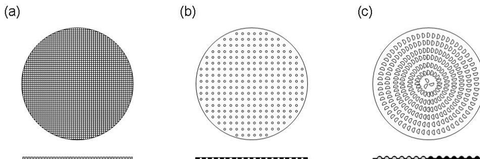
Figure 1: Distributor Designs (a) Dutch Weave Mesh; (b) Perforated Plate; (c) Punched Plate
