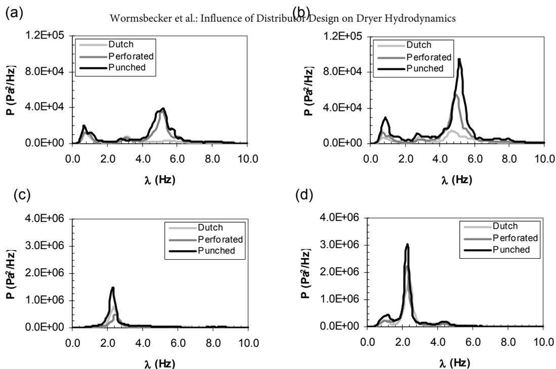
**Figure 6: Power Spectrum for 3.0 kg Loadings Dried at 1.5 m/s (a) 16 minutes into drying; (b) 32 minutes into drying; (c) 56 minutes into drying; (d) 88 minutes into drying**
