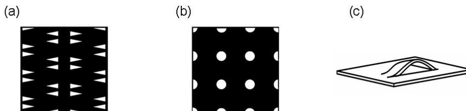
Figure 2: Details of Distributor Designs (a) Dutch Weave Mesh; (b) Perforated Plate; (c) Punched Plate
