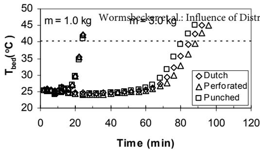
**Figure 3: Product Temperature Profile for Drying at 1.5 m/s**
