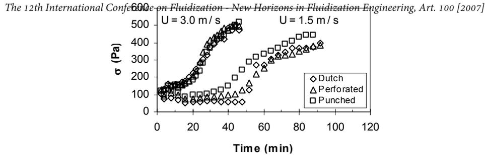
**Figure 5: Standard Deviation of Pressure Fluctuations for 3.0 kg Bed Loading**
