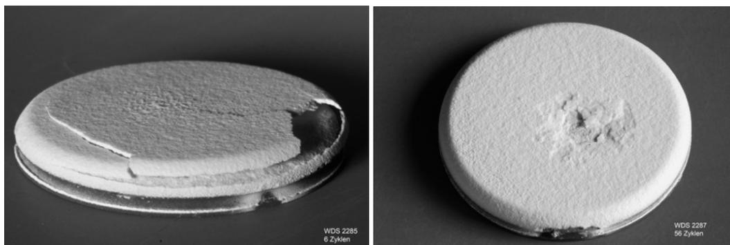
*Figure 1 – CMAS induced failure of TBC ceramic topcoats differing in modes of delamination and cycling lifetime correlated to specific load conditions.*
