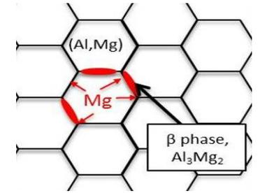
✓ Commercial Al-Mg alloy, strain hardened by 20% of cold work, 10 years Lab. conditions
