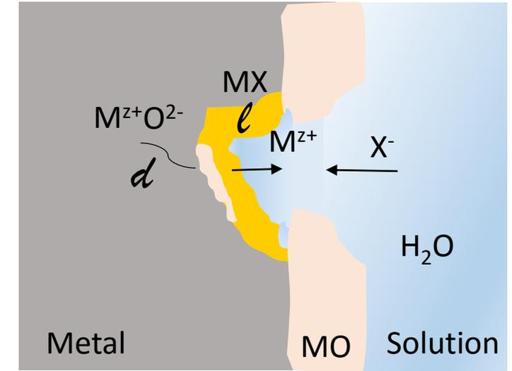
Very thin oxide film extends over the active surface on the pit bottom and then increases its thickness, resulting in complete repassivation.
