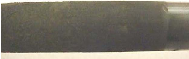
Fig. 3b Photograph of the probe with deposits focused at the mid-section of the heated test section.
