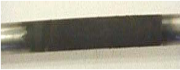
Fig. 3a Photograph of the probe with deposits (showing the clean surface at the inlet and outlet of the heated test section) after an LSB run.
