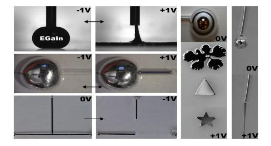
Figure 1 – Liquid metal (eutectic gallium indium, EGaIn) forms a surface oxide that can be controlled electrochemically to manipulate its shape.
