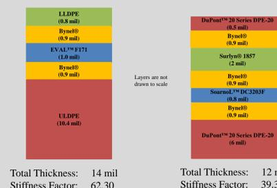
An optimized film structure would include a contact material that has a low extractable profile, such as DuPont™ 20 Series DPE-20, a more flexible EVOH such as SoarnoL™ DC3203F, and other tough layers such as Surlyn® 1857.
