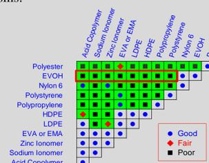
Grades within the DuPont™ Bynel® 4100 and 4200 series are widely used as tie layer resins for EVOH-PE structures.
