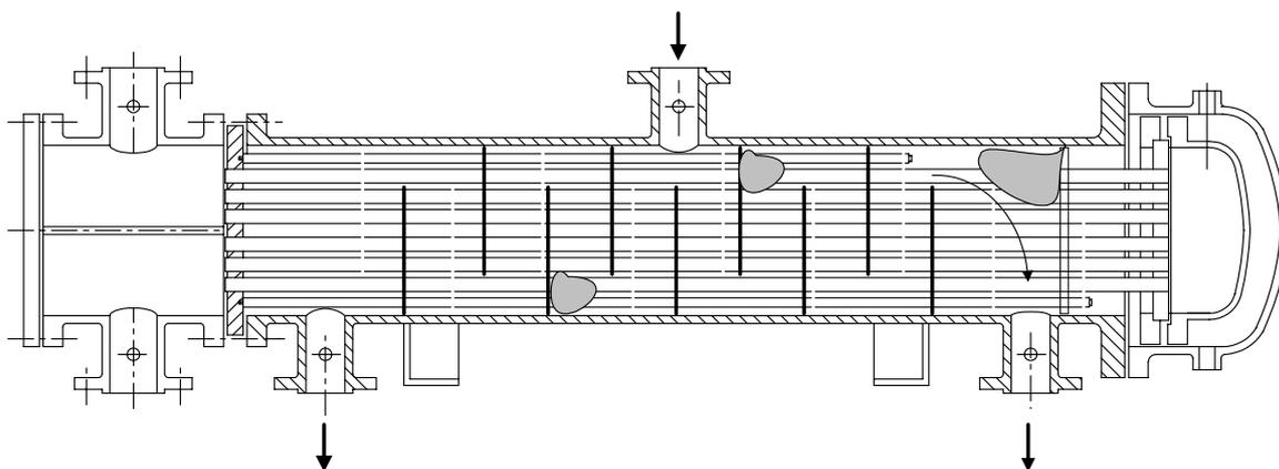
Fig. 1 Details of a typical shell-and-tube heat exchanger
