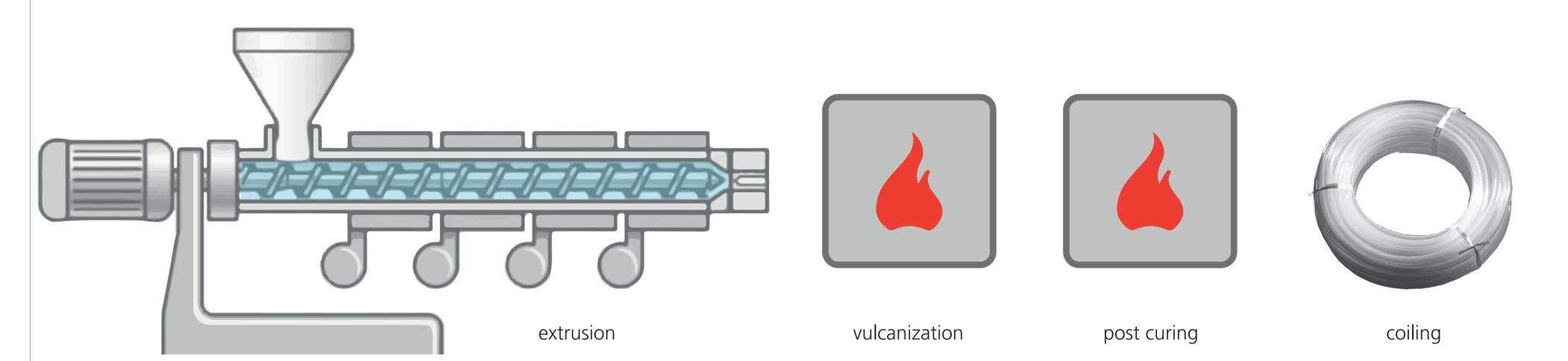
All silicones processed by RAUMEDIC are tested very comprehensively with several bio.-tox. tests including USP Class VI and ISO 10993. Furthermore post-curing after production is obligatory in order to achieve a save and high quality product.
