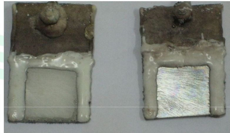
Appearances of Mn treated by chromate (Cr-Mn) (left) and \text{H}_3\text{PO}_4 (P-Mn) (right)
