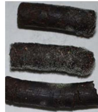
Pellets made from canola straw after 20 hours in humidity chamber, pellets made from untreated biomass (left), pellets made from torrefied biomass 0% binder (middle), pellets made from biomass with 5% binder (right).
