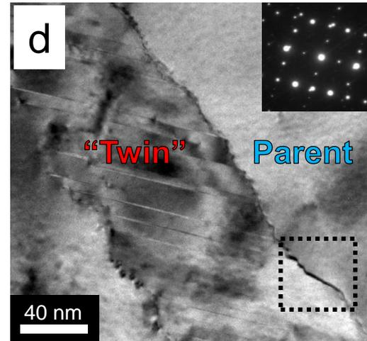
Larger grains in AZ31 Mg alloy sheet (30 mm × 30 mm × 22 mm) w/ equiaxed and strongly textured grains (average grain size ~34 μm). The compression loading was applied perpendicular to [0001] at a strain rate of  $10^3\text{s}^{-1}$  and a total strain of ~7%.
