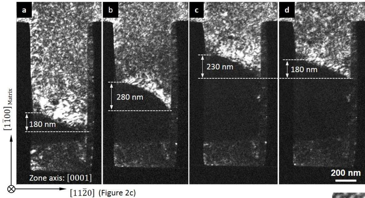
Cs-corrected STEM image of a Nano-milled <90 nm sample
