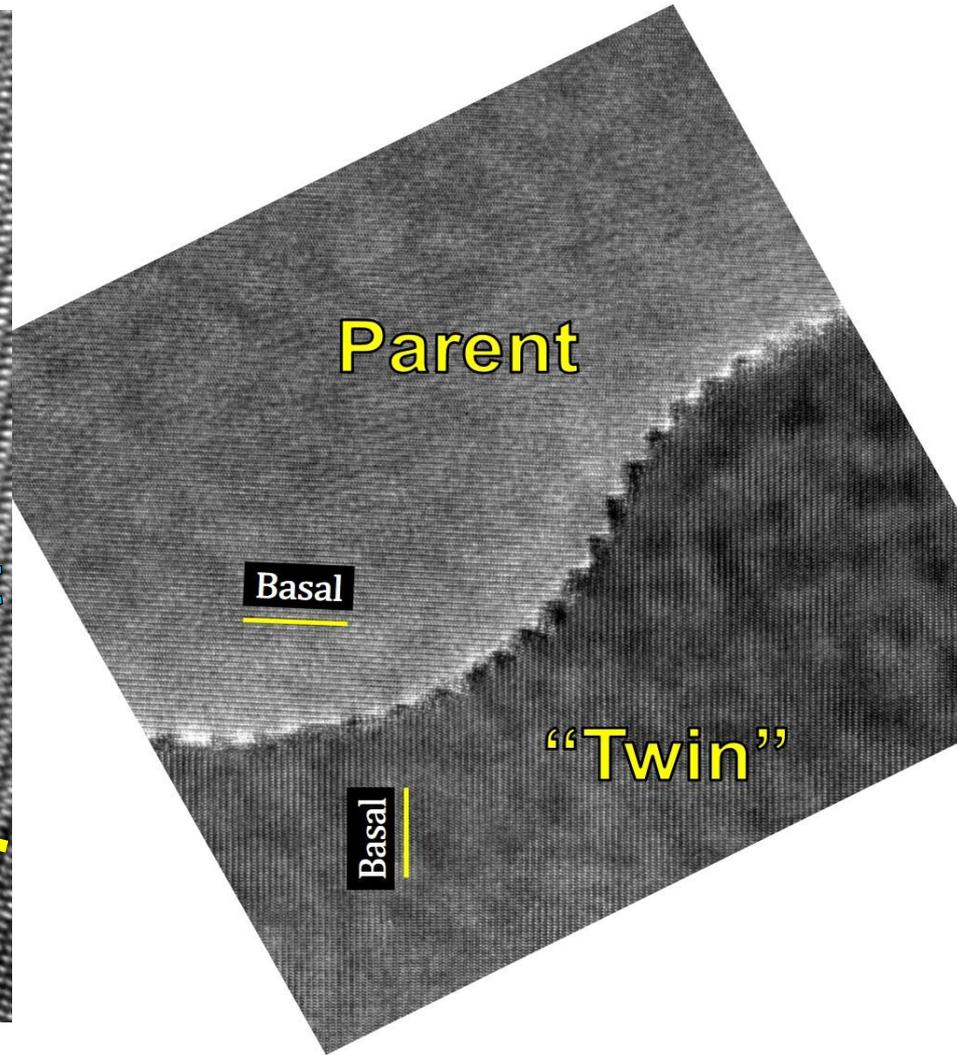
AZ31 Mg alloy sheet (30 mm × 30 mm × 22 mm) w/ equiaxed and strongly textured grains (average grain size  $\sim 34 \mu\text{m}$ ). The compression loading was applied perpendicular to [0001] at a strain rate of  $10^3 \text{s}^{-1}$  and a total strain of  $\sim 7\%$ . Note the **orthogonal steps**. This morphology is more obvious near twin tips.
