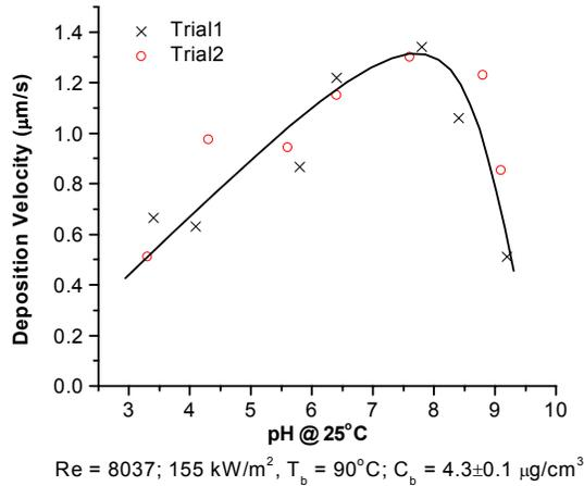
Figure 2. Variation of deposition velocity with pH<sub>25°C</sub>.
