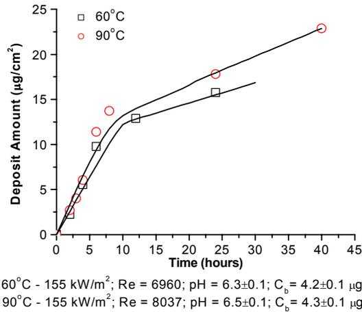
Figure 6. Variation of deposit with time at 155 kW/m<sup>2</sup> heat flux and two bulk temperatures.
