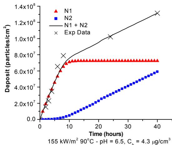
Figure 8. Modelling results applied to subcooled boiling condition.
