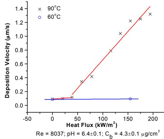
Figure 3. Variation of deposition velocity with heat flux.
