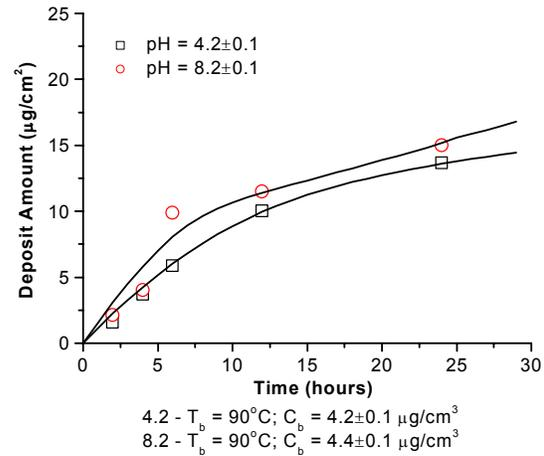
Figure 7. Variation of deposit with time at 155 kW/m<sup>2</sup> heat flux and two pH values.
