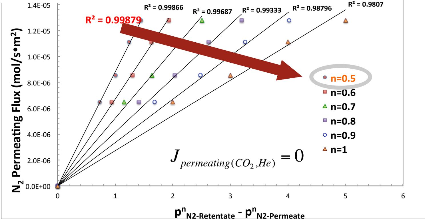
Similar to a Pd-based membrane for H<sub>2</sub> separation, N<sub>2</sub> molecules preferentially permeate through metallic membrane by the solution-diffusion mechanism
