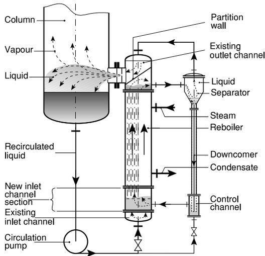
Fig. 4 Existing conventional reboiler retrofitted into self-cleaning configuration.
