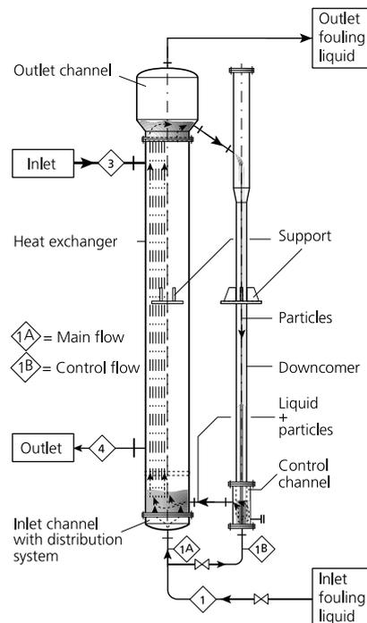
Fig. 2 Principle of self-cleaning heat exchanger with widened outlet channel.
