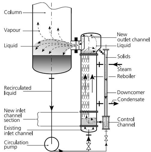
Fig. 5 Existing conventional reboiler retrofitted into self-cleaning configuration.
