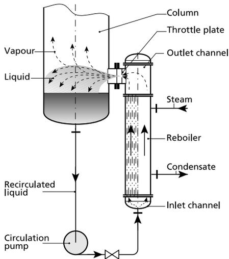
Fig. 3 Existing conventional reboiler.
