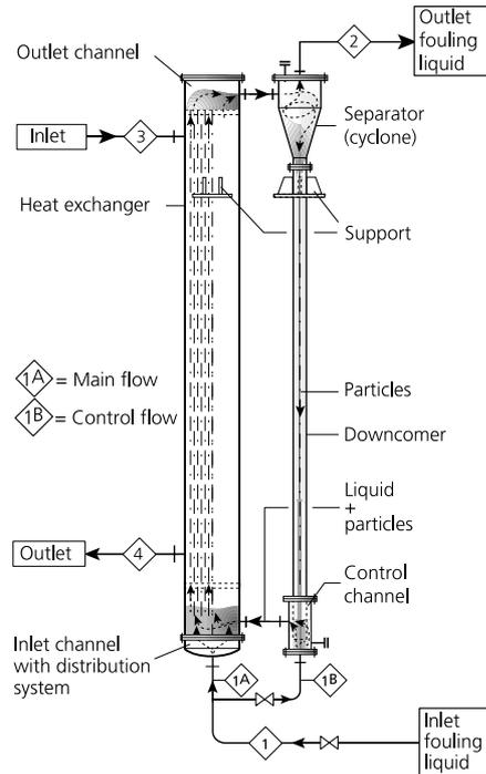
Fig. 1 Principle of self-cleaning heat exchangers with cyclone.
