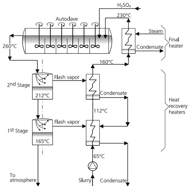
Fig. 6 Principle HPAL for laterite slurry
