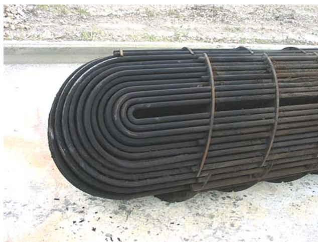
Fig. 10(b) Case 4: HELIX Bundle with Uniform Fouling
