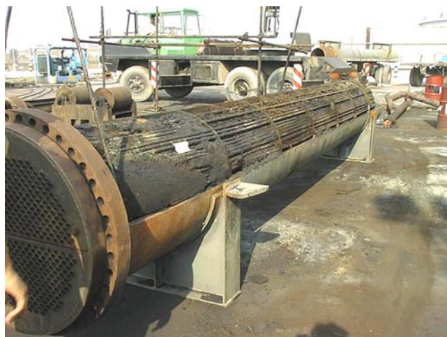
Fig. 10(a) Case 4: Segmental Bundle with Heavy Fouling
