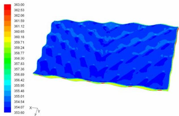
Fig. 4. The temperature field (K) when heat transfer was defined with the Constant wall temperature boundary condition and flow field was calculated with the RNG k- $\epsilon$  - turbulence model (Re = 2740, flow in z-direction).
