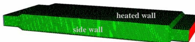
Fig. 2. 3D flat plate heat exchanger geometry with the computation mesh.
