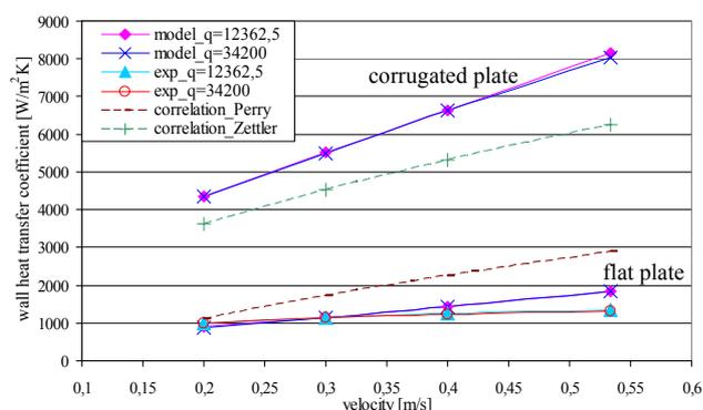
Fig. 9. Heat transfer coefficients as a function of velocity obtained with the experimental tests, and with the flat plate and corrugated geometry models, when Heat flux is used as a boundary condition.
