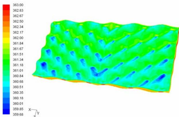
Fig. 6. The temperature field (K) when heat transfer was defined with the Convection boundary condition and flow field was calculated with the RNG k- $\epsilon$  -turbulence model (Re = 2740, flow in z-direction).
