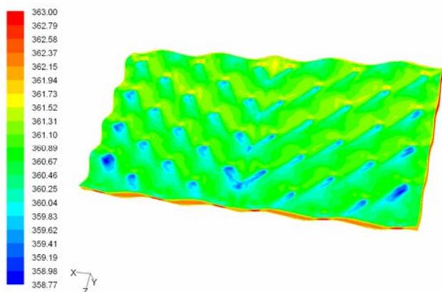
Fig. 5. The temperature field (K) when heat transfer was defined with the Heat flux boundary condition and flow field was calculated with the RNG k- $\epsilon$  -turbulence model (Re = 2740, flow in z-direction).
