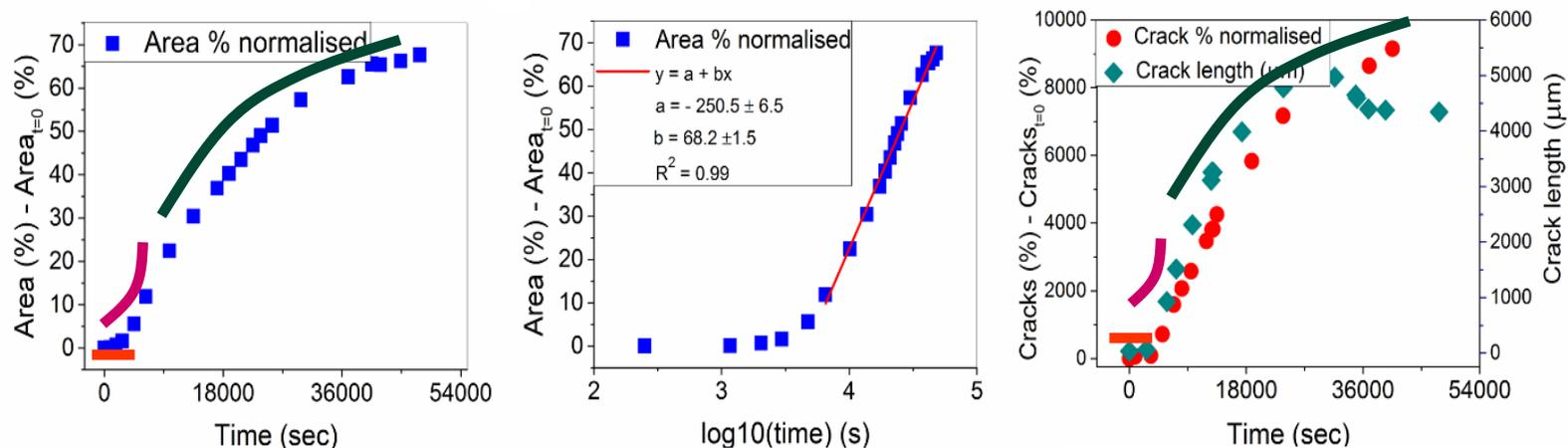
Sample area expansion and crack propagation follow a similar trend comprised of: **induction period**, **exponential area expansion and crack propagation** followed by and **logarithmic trend**.
