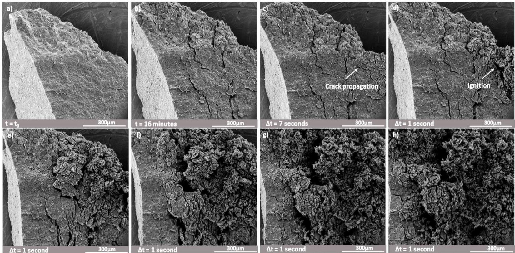
The SHS reaction in this sample propagates with a speed between  $150 - 500 \pm 50 \mu\text{m/s}$  across the sample.
