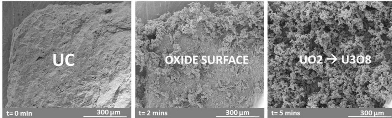
**10 Pa  $\text{O}_2$   $T = 800^\circ\text{C} \rightarrow$  oxidation not yet completed in 3 hours**
