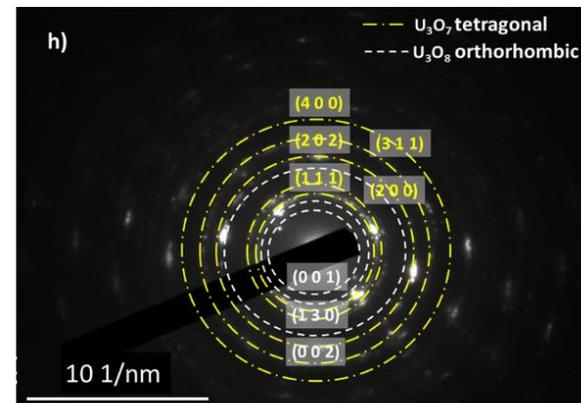
HRTEM analysis shows the oxide to be orthorhombic  $U_3O_8$  and tetragonal  $U_3O_7$ .  $U_3O_8$  transformation is triggered by ignition of UC which propagates as a SHS reaction.
