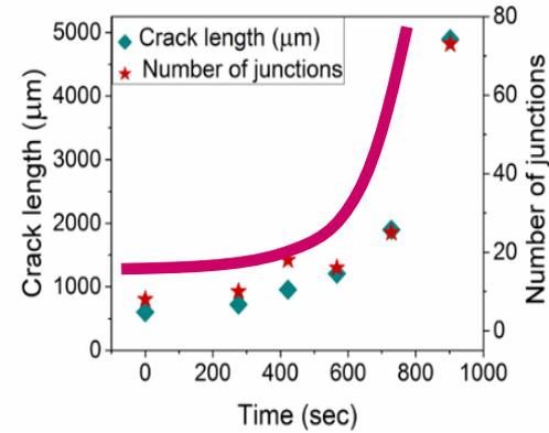
Sample area expansion, crack propagation crack length and number of junctions all follow an **exponential trend**. UC ignition is triggered by the fragmentation of the sample.
