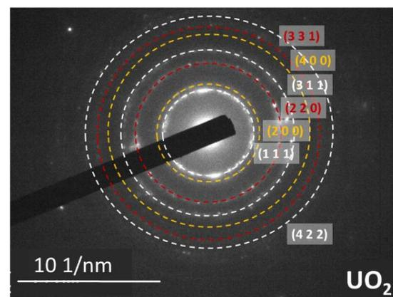
HRTEM analysis shows the oxide to be polycrystalline  $\text{UO}_2$
