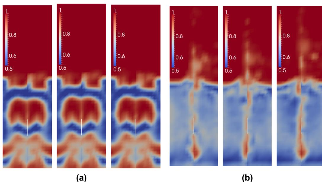
Figure 4. Snapshots of the voidage as a function of the Hamaker constant, respectively  $A = 0, 10^{-21}$  and  $10^{-19}$  J, in the bed for (a) the jet turned off and (b) the jet turned on. The snapshots are taken 1 s after the start of the simulation.
