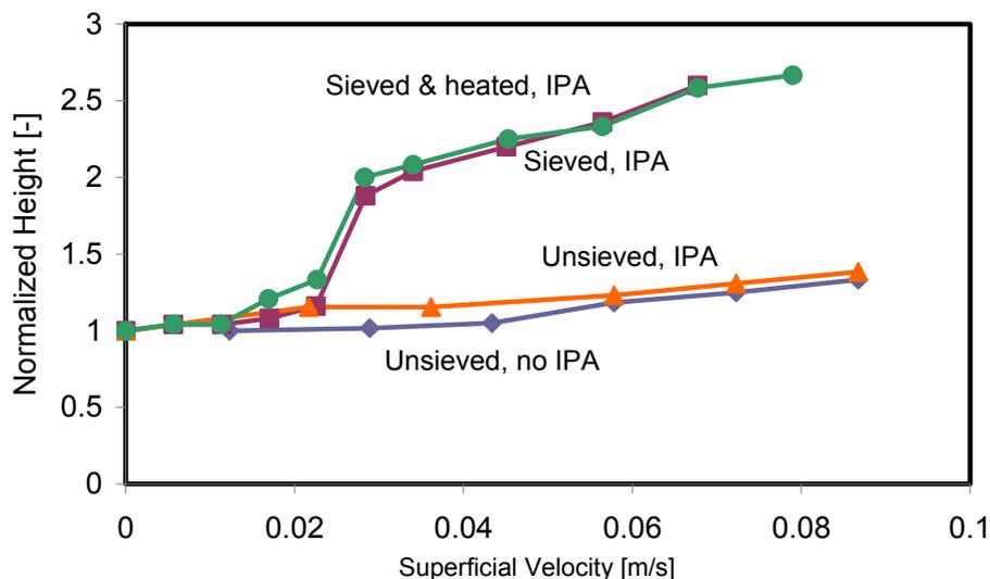
Figure 1. The effect of sieving, heating, and adding isopropanol (IPA) on the normalized bed height for the case without a microjet.
