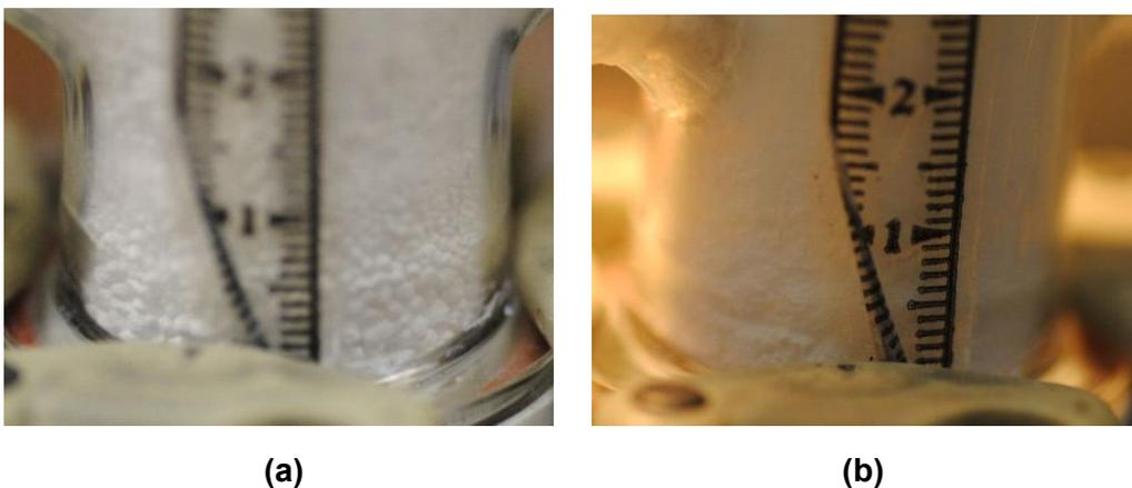
Figure 3. The powder in the bottom of the bed (a) before and (b) after processing with the microjet. While in (a) agglomerates are clearly visible, no agglomerates can be seen in (b).
