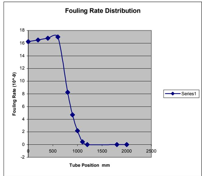
Figure 5. Development of fouling in unit having 80 tubes of 2500 mm length, fouling rate as function of position in tube
