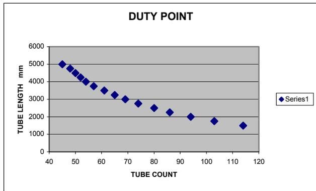
Figure 1. VTR Geometry, combinations of tube count and tube length providing Required Heat Duty
