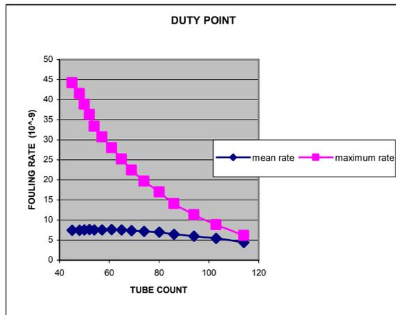
Figure 4. Fouling Rates as a function of design mean and maximum fouling rates as function of tube count for specified duty.
