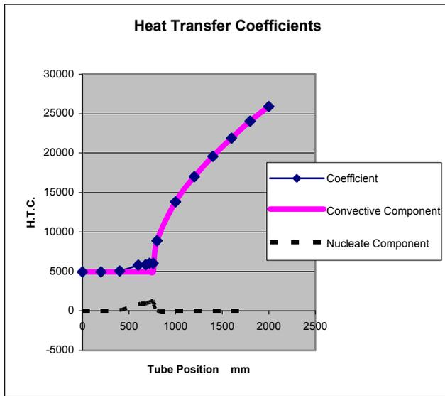
Figure 6. Local heat transfer coefficients in unit having 80 tubes of 2500 mm length
