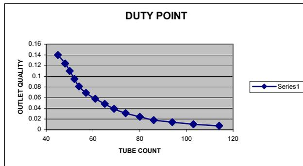
Figure 2. Effect of Geometry on Degree of Vaporisation outlet vapour mass quality for geometry providing required duty
