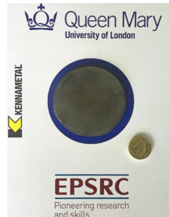
Figure 2 – \Phi 60mm flash sintered SiC sample
