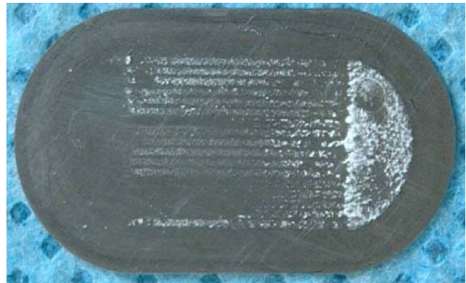
Figure 7: microstructured device and metallic foil (stainless steel) of the disassembled microstructured heat exchanger.
