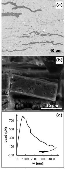
Figure 1 (a) SEM image of organic-rich shale (kerogen—dark gray, rock matrixlight gray), (b) SEM image of microcantilever beam after applying load, and (c) load-displacement curve from the micro-cantilever testing.
