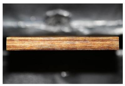
**Figure 1.** The cross-section of a well-consolidated glass fiber reinforced bioepoxy network.
