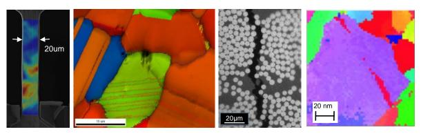
Figure 1: strain, stress and orientation maps of tensile, fatigue, fracture and twinning processes.
