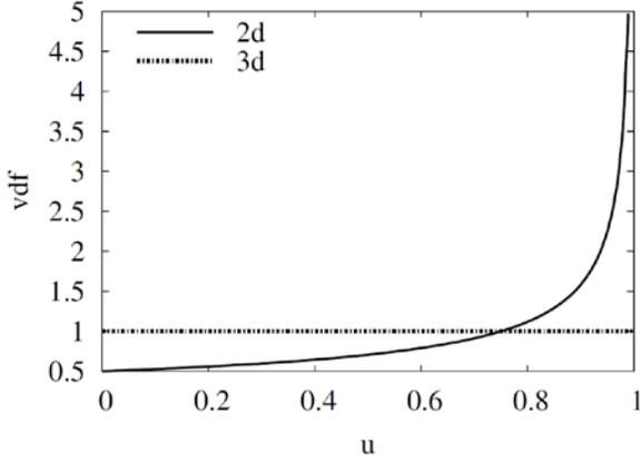
Figure 2: The velocity distribution function of the velocity parallel to the macroscopic flow direction, for the two- (Eq. 3) and three-dimensional (Eq. 2) Poiseuille flow (with  $u_0=1$ ).
