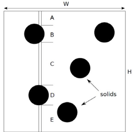
Figure 6: A simplified model of a highly porous two-dimensional system. Black circles represent solid grains. Segments A, C, and E are permeable to the flow.
