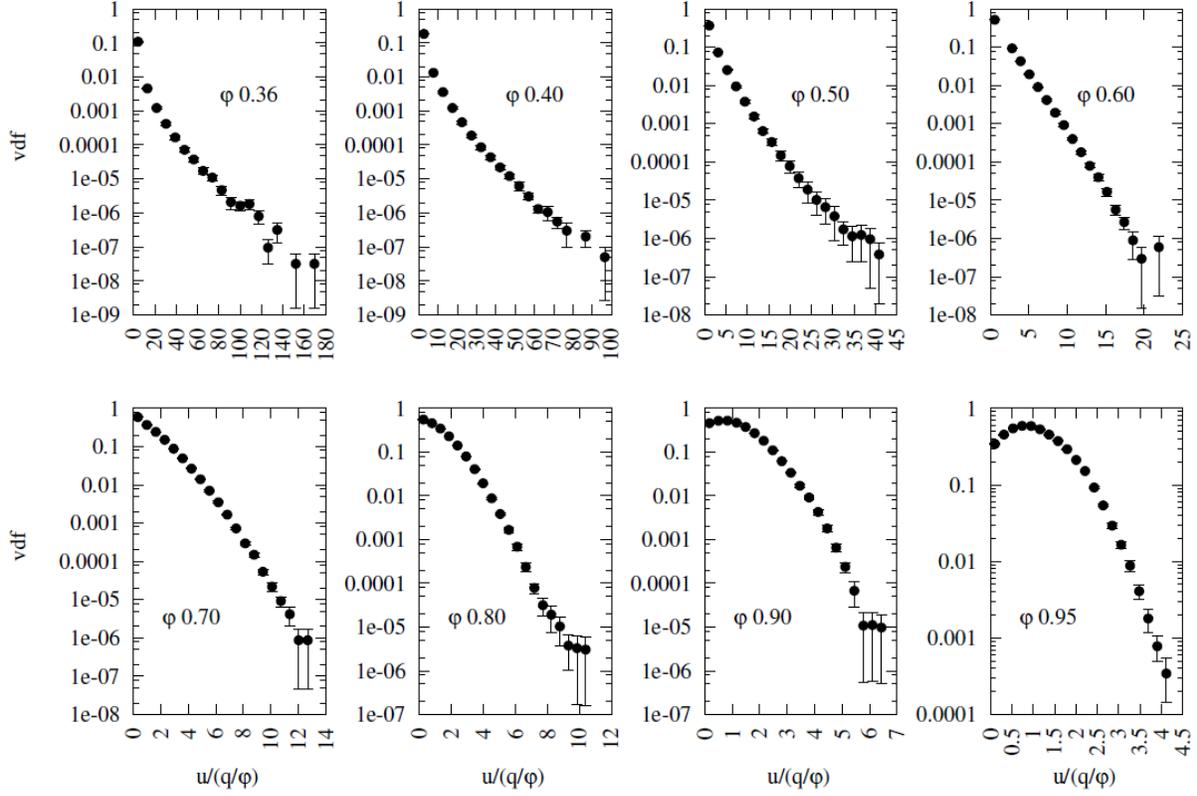
Figure 5: A semilogarithmic plot of the velocity distribution function for porosities ranging from  $\phi=0.36$  (left top) to  $\phi=0.95$  (right bottom). The error bars represent the standard error of the mean taken over 10 independent obstacle configurations at a given porosity. Note the variation of the axis scales.
