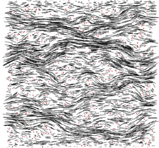
Figure 3: (Color online) Velocity vectors for  $\phi =0.99$ . The system size is  $1000 \times 1000$  and the diameter of each individual circular grain is  $a=4$  lattice units.
