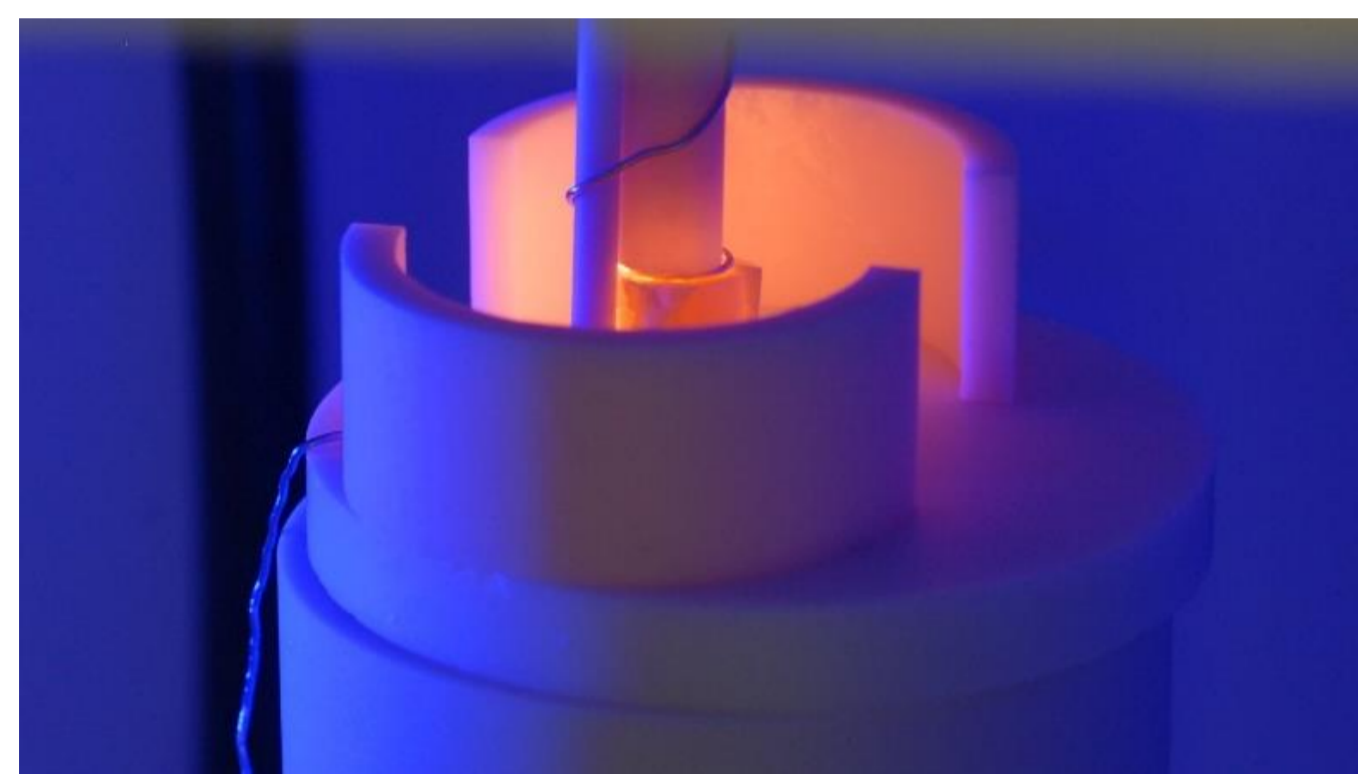
flashed sample in opened furnace at ~500 °C
