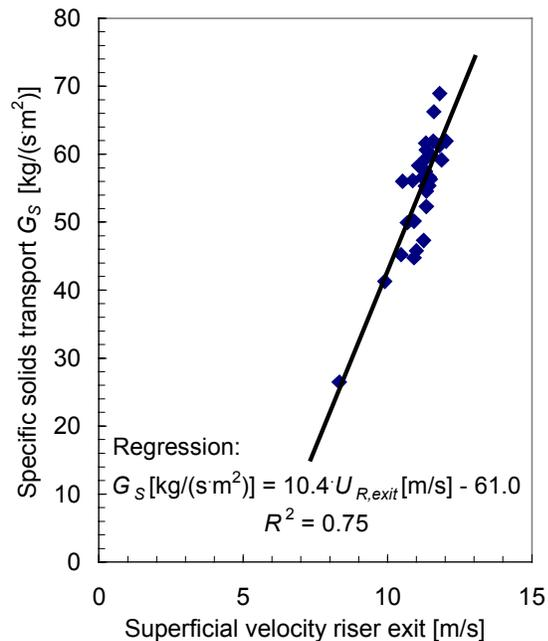
Fig. 3: Solids transport rate vs. riser exit velocity.
