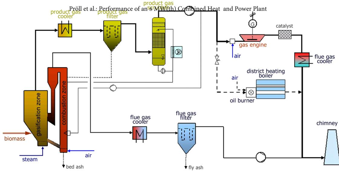
**Fig. 2: The 8 MW<sub>th</sub> biomass CHP plant in Guessing/Austria.**
