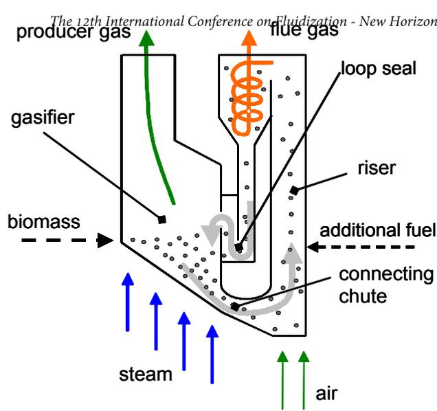
**Fig. 1: Dual bed steam gasification of solid biomass.**
