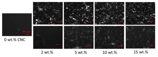
Figure 1 – Polarized light microscopy images of CNC/epoxy composites. Top: one-step mixing, bottom: two-step mixing [1, 2]. Lesser birefringence was observed for samples produced by two-step mixing, indicating that CNCs domains were smaller.
