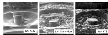
Pillars of 4  $\mu\text{m}$  diameter and 8  $\mu\text{m}$  height are fabricated (FIB) and compressed in different positions with respect to the near surface. The true stress-strain curves present a gradient on the yield stress. Pillars in single crystal deform in well oriented slip planes, contrary to the polycrystalline pillars, where deformation is completely homogeneous.
