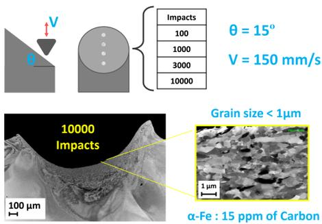
A pure Iron sample is impacted repetitively by a conical tungsten carbide tip. Four prints are created using a different amount of impacts. The angle and the impact velocity are controlled. The microstructure in the near surface is refined below a grain size of 1  $\mu\text{m}$ .
