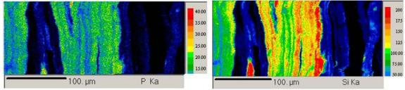
Figure 2 – EPMA P and Si mapping on fibers treated with Si and P containing precursor
